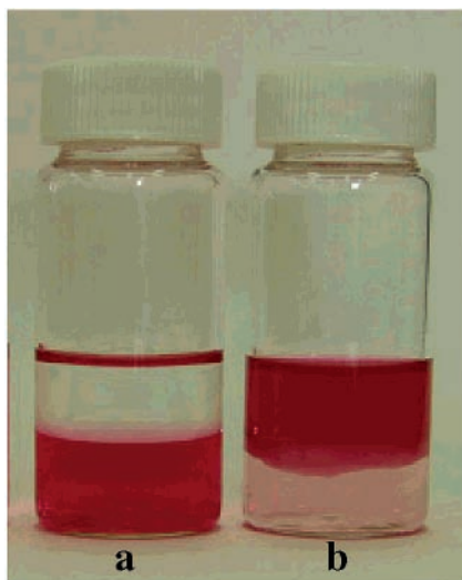
Figure 3. Migration of anthocyanin from the aqueous to hexane phase by the addition of AOT. (a) Before the addition of AOT. (b) After the addition of AOT. AOT (1 M) was added to 10 mL of biphasic hexane–water solution (1:1, v/v) where anthocyanin was solubilized in the water phase. The mixture was vortexed, and color transfer was observed.
